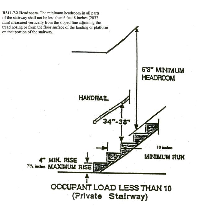
R311.7.4.1Riser height. The maximum riser height shall be 7<sub>3</sub>/<sub>4</sub> inches (196 mm). The riser shall be measured vertically between leading edges of the adjacent treads. The greatest riser height within any flight of stairs shall not exceed the smallest by more than 3/8 inch (9.5 mm).
